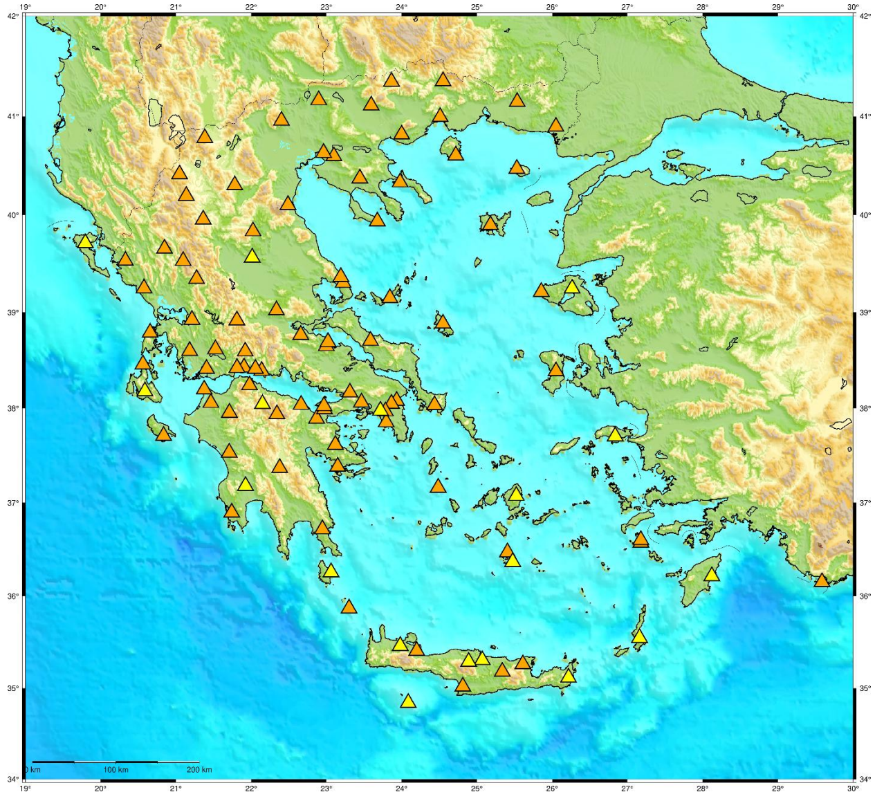
Figure 1: Station distribution of the Hellenic Unified Seismic Network (HUSN) used in this study. The orange triangles represent broadband stations where only data from Z component are utilized, while the yellow triangles represent stations that we use data from all three components.
